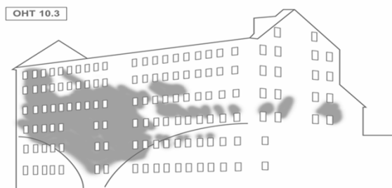
Figure 10.5 V-shaped smoke damage evident when a burnt building is viewed as a whole from the outside
